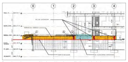
Section showing the recostruction of the plaza and the realignment of building and plaza levels
